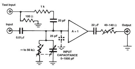
Fig. 1. Simplified Schematic of the Model 113.
