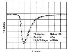
Fig. 1. Typical Anode Output with a Burle 8575 Photomultiplier Tube.
