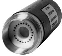
The ORTEC Model 265A Photomultiplier Base is a mechanical assembly and a resistive voltage divider network, with appropriate capacitive decoupling, for operation of 12-stage photomultiplier tubes (PMTs). It is particularly suited to applications requiring fast timing or single photon counting. The Model 265A accommodates the following types of PMTs.
