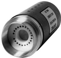
The ORTEC Model 265A Photomultiplier Base is a mechanical assembly and a resistive voltage divider network, with appropriate capacitive decoupling, for operation of 12-stage photomultiplier tubes (PMTs). It is particularly suited to applications requiring fast timing or single photon counting. The Model 265A accommodates the following types of PMTs.
