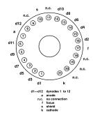
Fig. 2. Pin Assignments.
