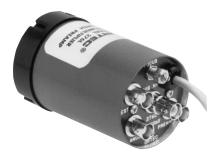
The ORTEC Model 276L Low-Power Photomultiplier Tube Base and Preamplifier incorporates an integral low-noise preamplifier, a PMT base with a low-power voltage divider network, and a focus control for optimum performance in scintillation detector applications. The unit is ideally suited for use with Nal(TI) detectors.
