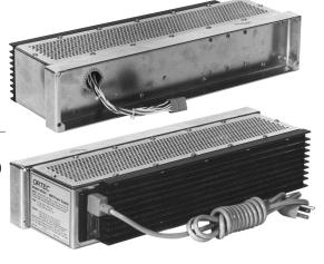
**CIRCUIT PROTECTION** Input power line fused. Power supply is automatically cut off by an internal switch if the temperature exceeds a maximum safe limit. Output current foldback limiting with automatic recovery when demand is removed.
