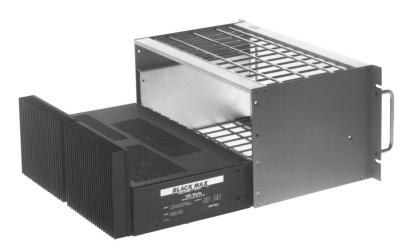
An external slide switch allows selection of either 115 or 220 V AC as the power input. By changing pins on an internal connector, this selection can be altered to 100 and 200 V AC. An international standard IEC power connector permits power cords and plugs that meet local electrical standards to be used for the input power. Control of the primary power is provided by the On/Off switch on the NIM bin control panel.
