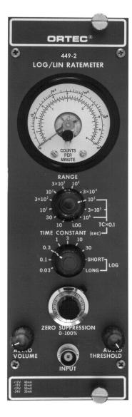
The ORTEC Model 449 Log/Lin Ratemeter provides two modes of operation: linear and logarithmic. The linear mode has 11 full-scale ranges from 10 to 10° counts/sec in 1-3-10 steps. The 5-decade log mode covers the range from 10 to 10° counts/sec in a single span. These selections permit logical operation of the instrument when measuring low, medium, or high steady pulse rates or when monitoring rates that vary through a wide range.
