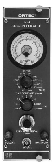
The ORTEC Model 449 Log/Lin Ratemeter provides two modes of operation: linear and logarithmic. The linear mode has 11 full-scale ranges from 10 to 10<sup>6</sup> counts/sec in 1-3-10 steps. The 5-decade log mode covers the range from 10 to 10<sup>6</sup> counts/sec in a single span. These selections permit logical operation of the instrument when measuring low, medium, or high steady pulse rates or when monitoring rates that vary through a wide range.
