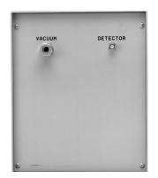
The ORTEC Model 808 Vacuum Chamber provides a quick and convenient way to measure the alpha and beta activity of environmental samples. It accommodates a wide range of sizes of samples and detectors. The chamber can accept sample trays measuring up to 10.8 x 14 cm (4.25 x 5.5 in.), with nominal sample size 10 cm (4 in.) in diameter.
