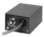
The ORTEC Model 9301 low-noise, fast-rise-time Preamplifier has been designed for use with photomultipliers, electron multipliers, and other detectors employed in photon counting, ion counting, or fast-timing applications. When connected to the detector, the 50- $\Omega$  input resistance of the Model 9301 provides a load resistance for the detector output current pulse.
