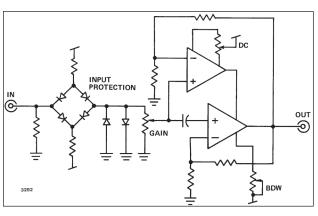
The Model 9305 Fast Preamplifier Circuit.
