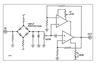
The Model 9305 Fast Preamplifier Circuit.
