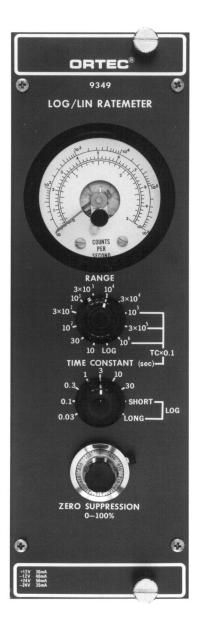
Designed for photon or ion beam applications, the ORTEC Model 9349 Log/Lin Ratemeter provides two modes of operation: linear and logarithmic. The linear mode has 11 full-scale ranges from 10 to 10<sup>6</sup> counts/s in 1-3-10 steps. The 5-decade log mode covers the range 10 to 10<sup>6</sup> counts/s in a single span. These choices permit optimum measurement of low, medium, or high steady pulse rates or monitoring of rates that vary through a wide range.
