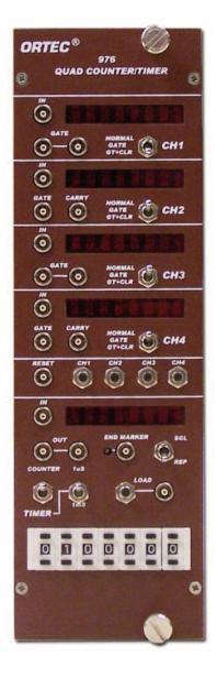
The 976 has four independent 8-digit counters each with their own display and can accept up to 250-MHz input rates. These counters can be cascaded to increase the word length to 16-digits for two counters, and
