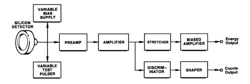
Fig. 1. Block Diagram of A-PAD A-576 Alpha Spectrometer.
