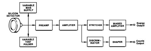
Fig. 1. Block Diagram of A-PAD A-576 Alpha Spectrometer.
