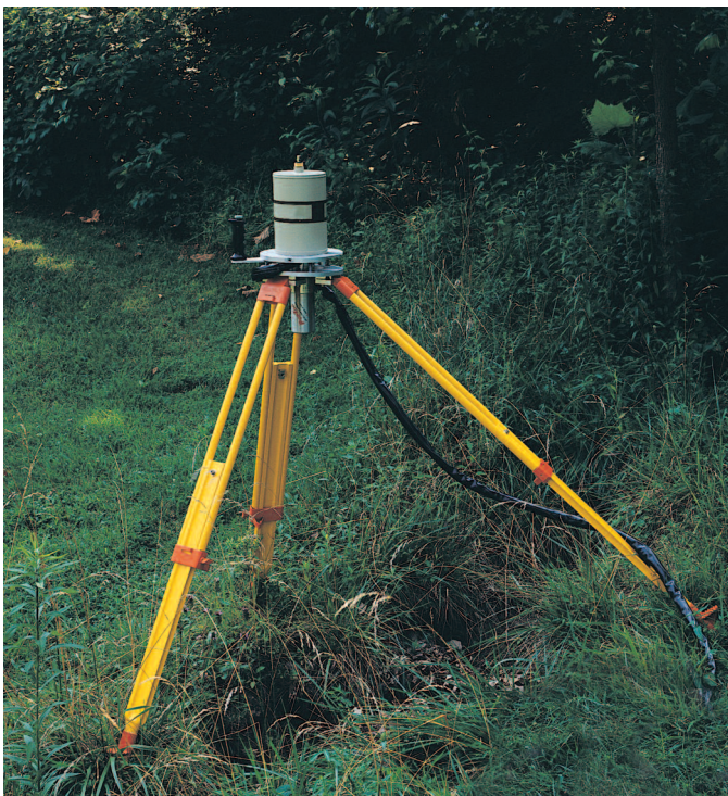
M-1-T1 Tripod with MG4 Gamma Gage Detector.
