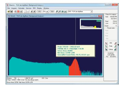
When viewing a live detector, the spectrum view is updated in real time and provides current spectral data, live peak calculations, and hardware properties — even for remote instruments connected to different computers on the network. Viewing spectrum peaks, library energies, or regions of interest is simple with the convenient side panel buttons.
