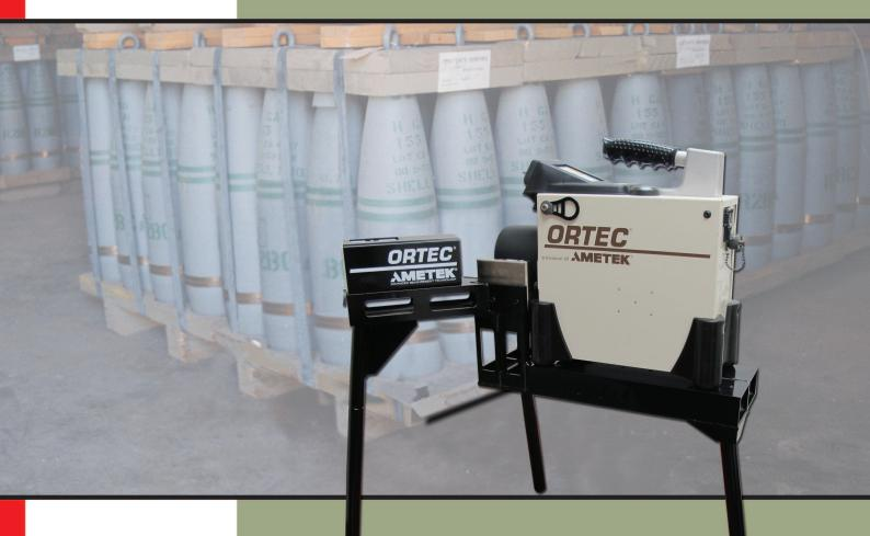
Portable Isotopic Neutron Spectroscopy System for the Identification of Chemical Warfare Agents, Explosives, and Toxic Industrial Chemicals without the need for Liquid Nitrogen.
