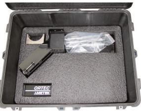
All of the system components fit into two ruggedized cases designed to handle the shock and vibration of impacts during movement and handling.
