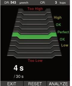
In Easy ID mode, the RADEAGLET-R acquires a spectrum. The screen at left is used to find an optimal position to ID the source. The user can preset duration if desired, then analyze and save the results. During the acquisition, an on-screen chart instructs the user to find the best distance between the instrument and the source in question. The nuclides identified will be displayed. The recorded spectrum and the analysis results are saved to an internal SD card in ANSI N42.42 format.
