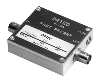
The Model VT120 Fast-Timing Preamplifier is a high-performance, wide-bandwidth preamplifier designed for boosting very fast linear signals from microchannel plates, photomultipliers, electron multipliers, silicon detectors, and other detectors used in fast timing applications. The rise time on all versions is <1 ns with a 5-V output, enabling excellent timing resolution.
