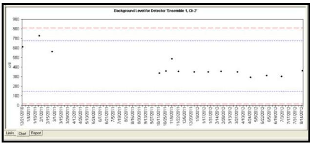
Figure 8. The QA Control Chart for Detector Background
