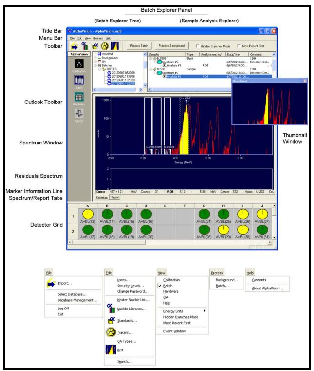
Figure 2. Batch Mode Screen Features and Menus
