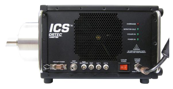
Figure 2. Connector Panel.
