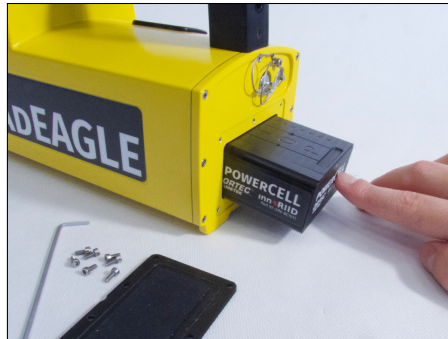
Figure 137: Inserting the POWERCELL
