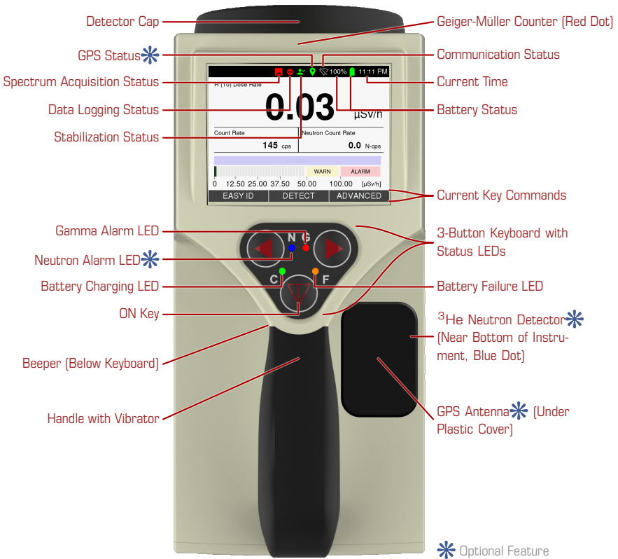
Figure 1: Annotated top view of the RAD EAGLE instrument
