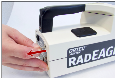
Figure 129: Pulling the protection of the power connector
