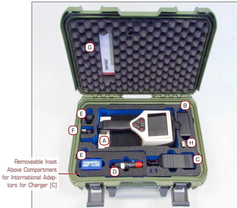
Figure 5: The RAD EAGLE in an optional watertight case
