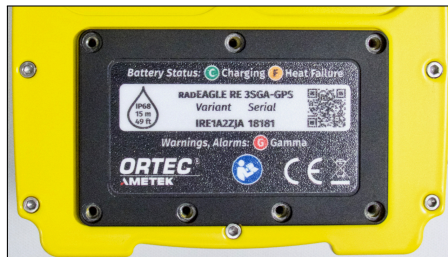
Figure 139: Correct placement of the battery cover plate
