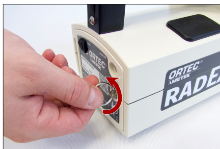
Figure 130: Opening the rear latch of the RAD EAGLE
