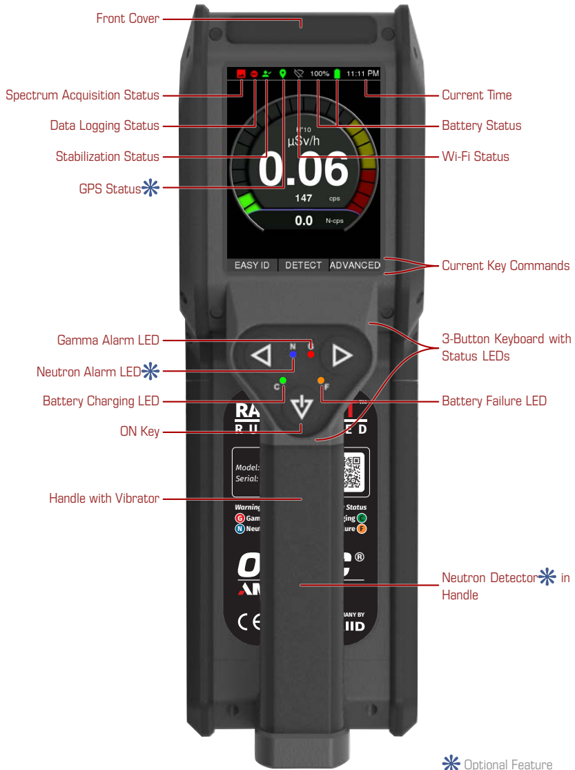
Figure 1: Annotated top view of the radEAGLET-R instrument
