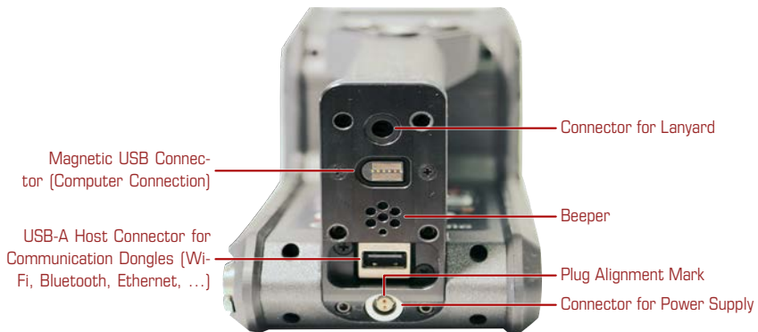
Figure 4: Rear view of the RAD EAGLET-R
