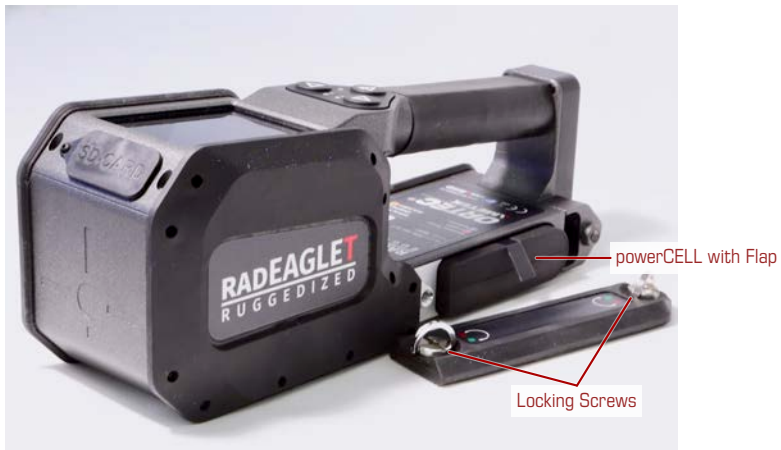
Figure 130: POWERCELL in compartment with cover removed
