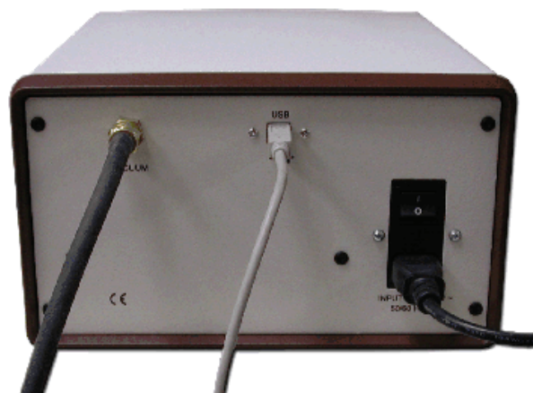
Rear of the Alpha Duo unit - requires just 3 inputs
