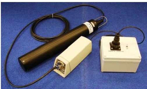
Figure 2 - Housing with MicroNomad & external battery pack
