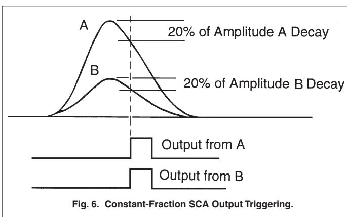
Fig. 6. Constant-Fraction SCA Output Triggering.
