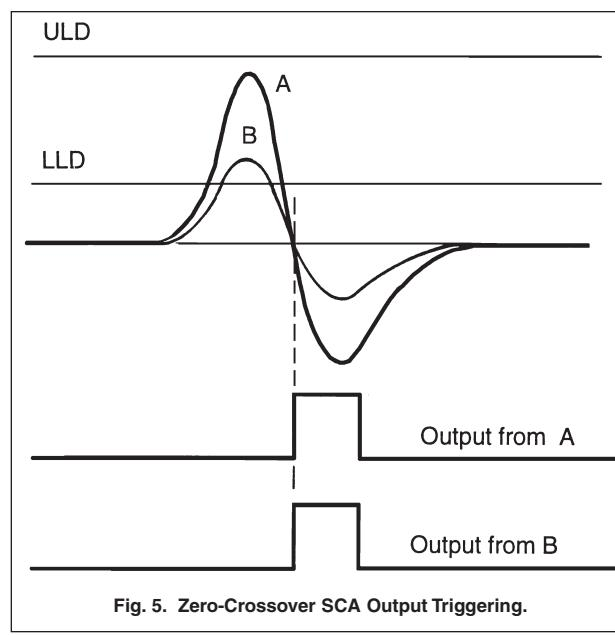
Fig. 5. Zero-Crossover SCA Output Triggering.
