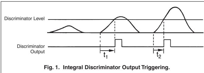
Fig. 1. Integral Discriminator Output Triggering.
