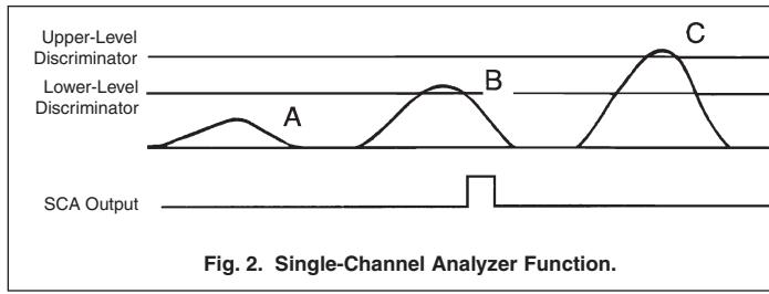
Fig. 2. Single-Channel Analyzer Function.
