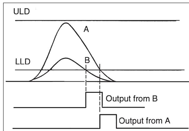
Fig. 3. Non-Timing SCA Output Triggering.
